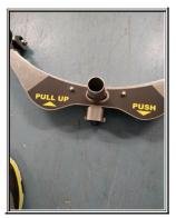
**Improvement 5.** New designed squeegee locking system. The squeegee assembly can be lifted and lowered easily by using your foot. (Below)
